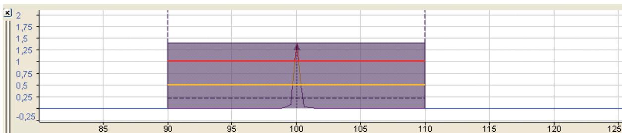
The most important parameters of the frequency bands and of the spectrum are shown with dotted and colored lines. You are shown the respective values when you position the cursor on the lines (hovering).
