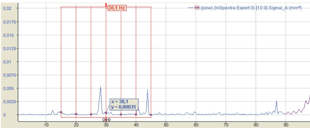
The above figure shows an interactive marker with 3 sidebands and offset of 3 Hz each.
