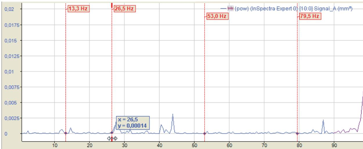
The above figure shows an interactive marker with 1 harmonic component below and 2 harmonic components above the marker frequency of 26.5 Hz.
