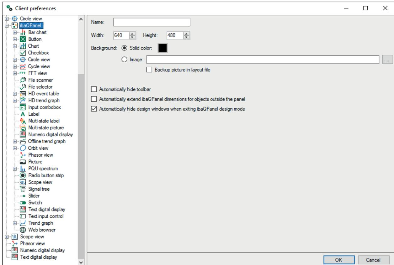
As described in [ibaQPanel](#), page 114, the *ibaQPanel* view is the base for an HMI-like screen design. Beside some special QPanel objects, like multi-state label, multi-state picture, button, label, bar chart, gauge panel and text input control, you can add all other types of views to a QPanel view. Consequently, there are preferences and properties settings for these objects available within the QPanel preferences and properties.
