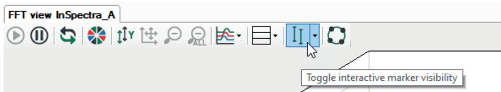
When activating for the first time, the marker is displayed at the position 1 Hz. Every time the marker is switched off and on again, it memorizes the last position.
