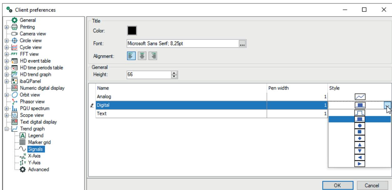
In this dialog you can generally define how the curves should be initially displayed. The default setting for curves of analog values is a simple line (line thickness 1), and for digital signals a filled area. Text signals will be displayed in standard font.
