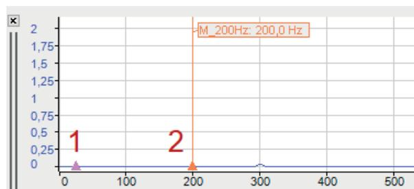
The example above shows a collapsed marker (1) and a normal marker (2).
