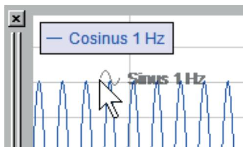
3. The result: two signals, each with its own Y-axis.
