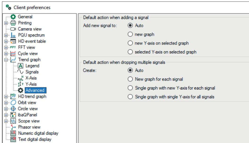
The default behavior is "Auto". If you add a signal with no key combination pressed, a new graph and a new Y axis will be created for the signal. If you hold the <Ctrl> key while adding a signal, a new Y axis is created in the currently selected graph chart and the signal is added to that new Y axis. If you hold the <Shift> key while adding a signal, the signal is added to the currently selected Y axis.
