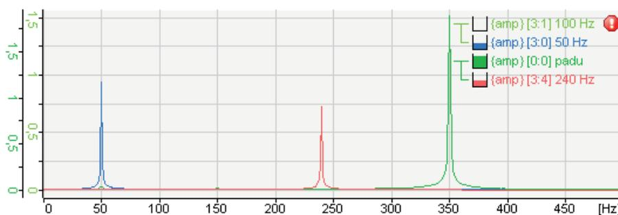
The legend has a drag & drop function. This way, a spectrum can be laid upon different value axes. While dragging the spectrum, an arrow appears in the value axis tree pointing to the tree that will contain the spectrum when it is dropped. If a spectrum is not dropped inside a legend row, the spectrum will be laid upon a new axis.
