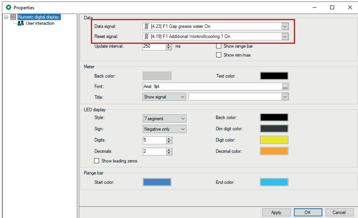
Preferences and properties of digital displays are basically the same except for the signal selection. Data signal and reset signal selection is available in the "Properties" dialog only (red frame in the picture above).
