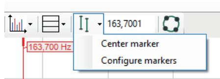
Click on the arrow symbol at the marker button in the tool bar and then on "Center marker."
