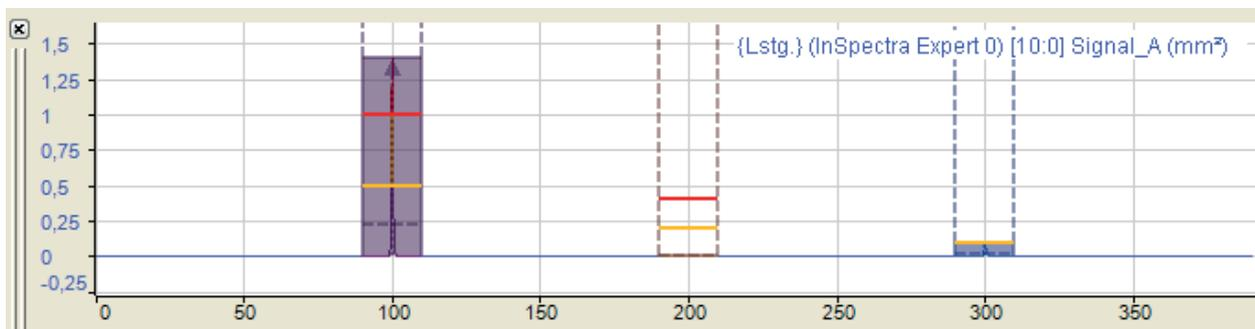
In the figure above the display shows three different frequency bands and at least a part of the spectral graphs from the main window. You can add additional graphs by dragging and dropping them from the main window or from the signal tree via drag & drop. The displays are linked so that all graphs in the small spectral display can also be seen in the main window.
