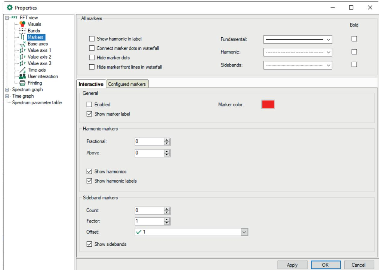
Harmonic markers always have a frequency that corresponds to an integer multiple of the main marker. For the harmonic markers, determine the requested number of the harmonic components below and above the current marker frequency. For the harmonic frequencies, further lines are displayed. Additionally, in the "Markers" branch, enable the option "Show harmonic labels" to display the frequency values on the markers.
