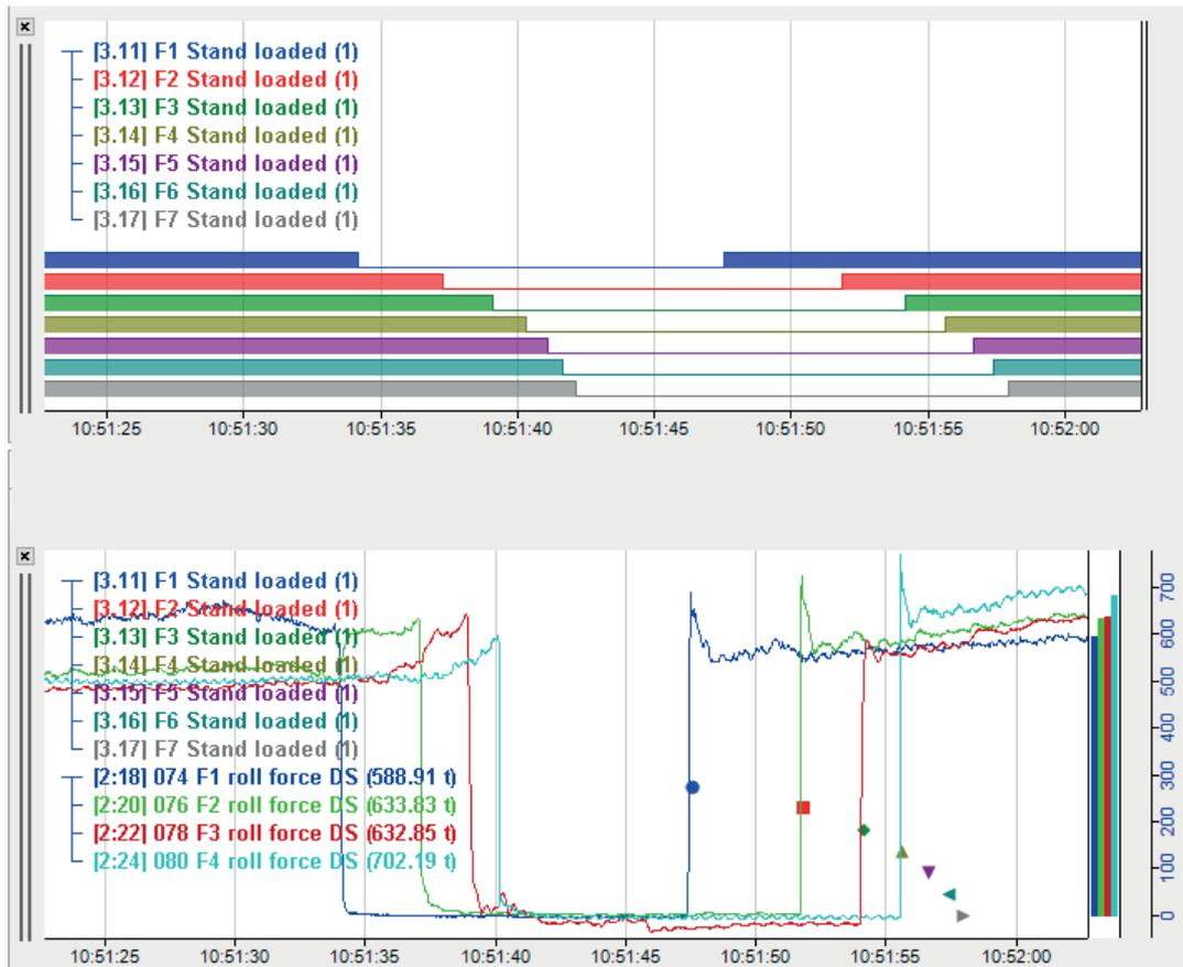
The symbolic style can be useful if the trend display would be overloaded in the standard style, especially when digital and analog signals are presented mixed.
