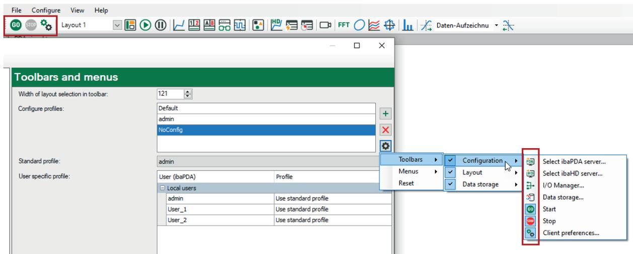
In the configuration toolbar section in the upper left corner, the buttons for server selection, I/O Manager and data storage configuration are missing.
