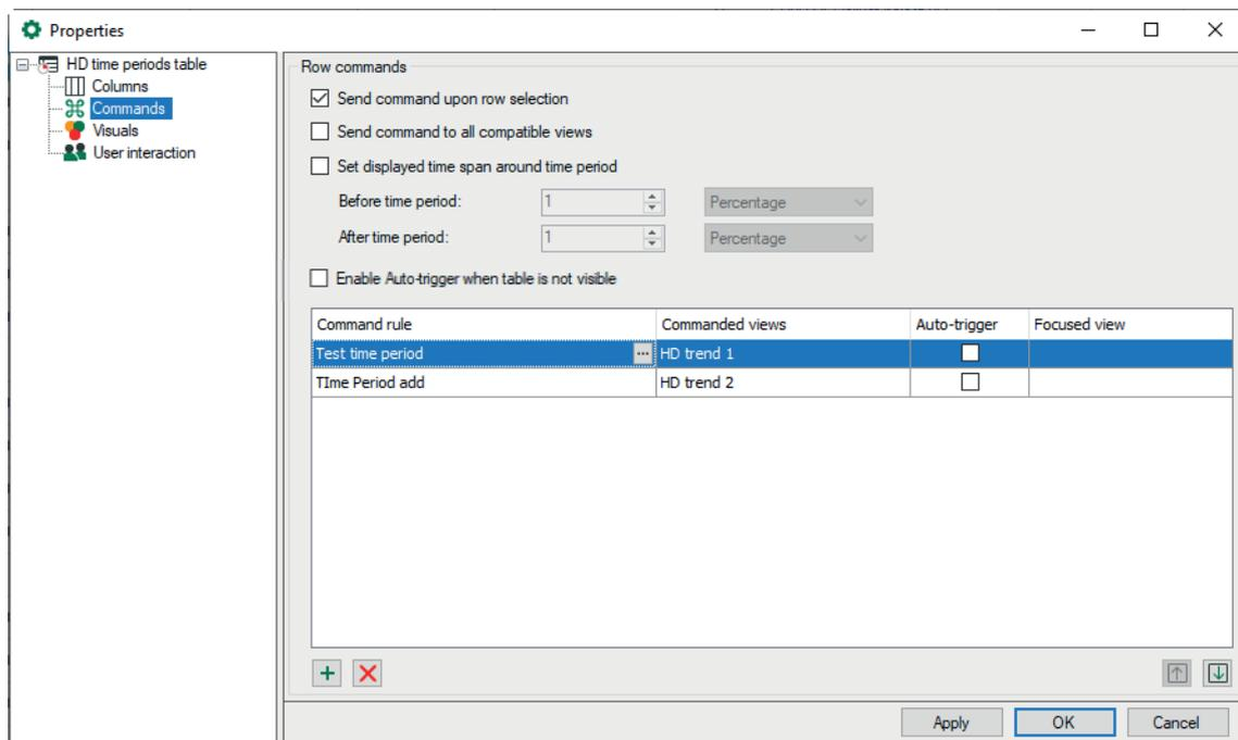
The *Send command to all compatible views* option is enabled by default. This means that when you double-click on a row in the table, all HD trend graphs show the selected time period. In this case, the command rules are disabled.
