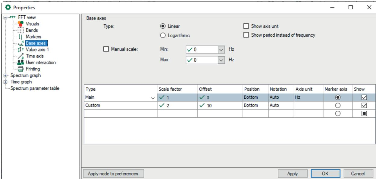
The figure above shows the properties of the base axes in the FFT view. By default, the scaling values are automatically determined. However, you can also make a manual specification.
