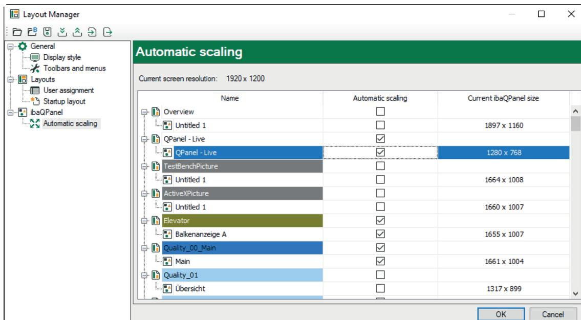
The scaling is carried out when opening *ibaPDA* on a screen with a different resolution. It also works on the fly if you drag the window to another screen with a different resolution.
