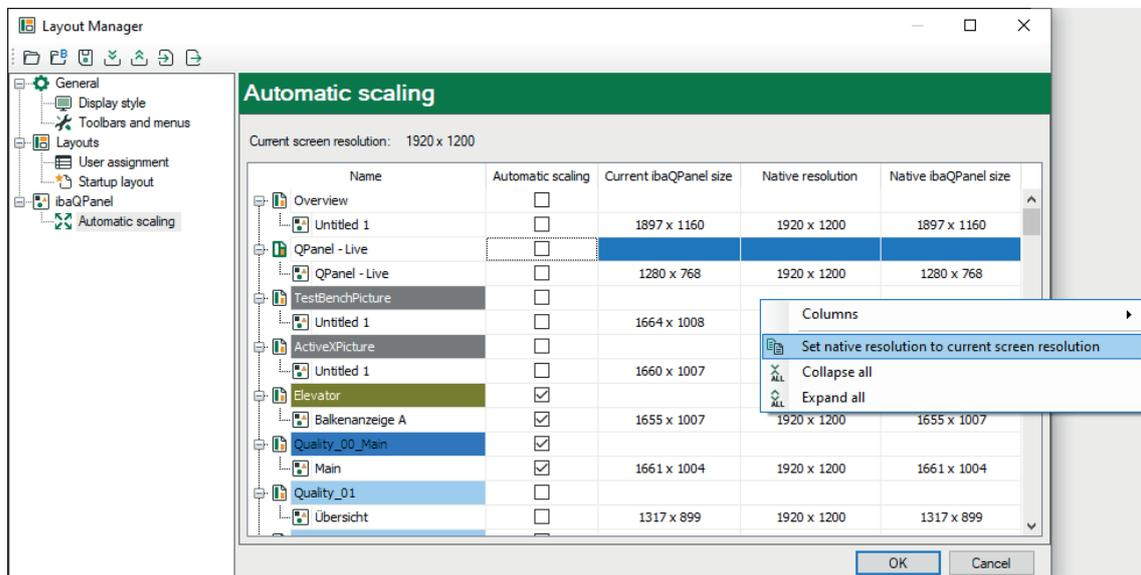
When you open an existing layout with an *ibaQPanel* window for the first time in the new version, the native resolution is initialized to the current screen resolution and the native size to the current size.
