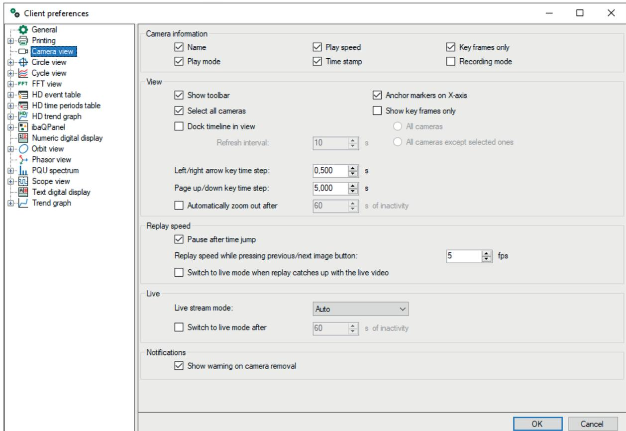
*ibaPDA* uses the same software components for the camera views like the *ibaCapture* Player. Thus, you can set up the same properties and features in the preferences of the camera view like you do in the properties of a camera in the *ibaCapture* Manager.
