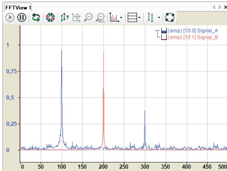
You can enable an interactive marker that you want to use to read frequency values and the associated amplitudes along the X-axis.
