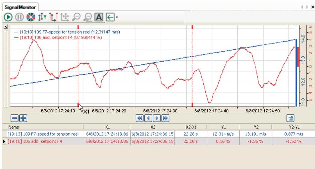
In pause mode, there are two markers, i.e. X1 and X2, available in the graph. You can move the markers individually in order to check the Y values and differences between the X and Y values of the markers.
