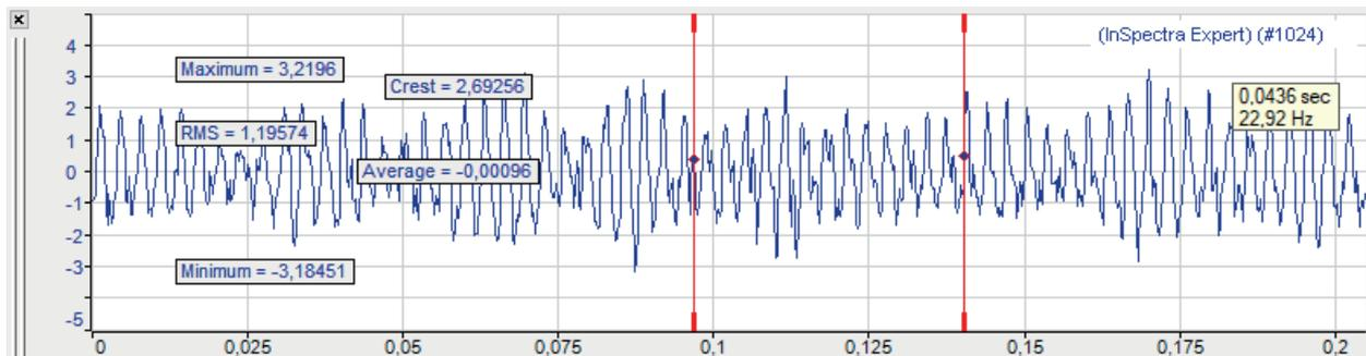
If the averaging function was enabled in the calculation settings of the profile, then the display shows the time signal of the last internal FFT calculation. The displays of the FFT results in the main window and frequency range, however, are also based on prior values of the input signal.
