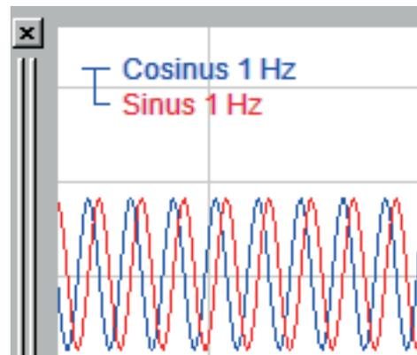
7. If you want to separate signals, just click on the corresponding signal in the legend and drag it into the free area of the display window's X axis. A new graph is opened with that signal.
