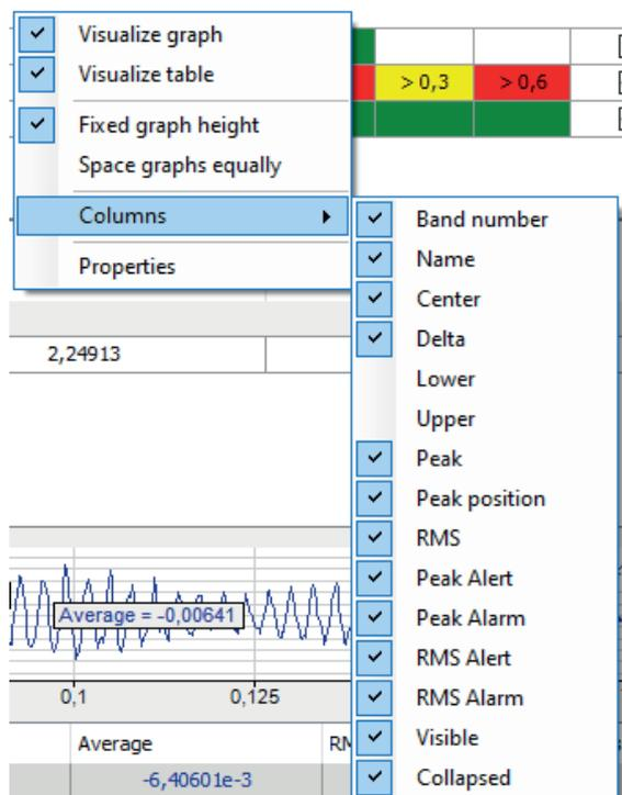
In every parameter column, the displayed values can be sorted by clicking on the table header. A triangle in the header indicates whether the sorting direction is ascending or descending. The order is automatically re-sorted if the order changes during acquisition.
