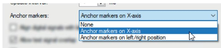
If the *Anchor markers* option is disabled (*None*), the markers will remain at the same pixel while moving the X-axis and are positioned on a new time stamp, e. g. when dragging or panning.
