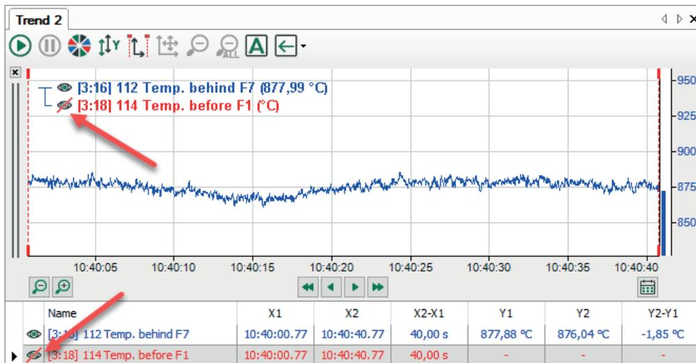
If a signal is hidden then the signal bar is also empty and no marker or actual values are displayed in the signal table.
