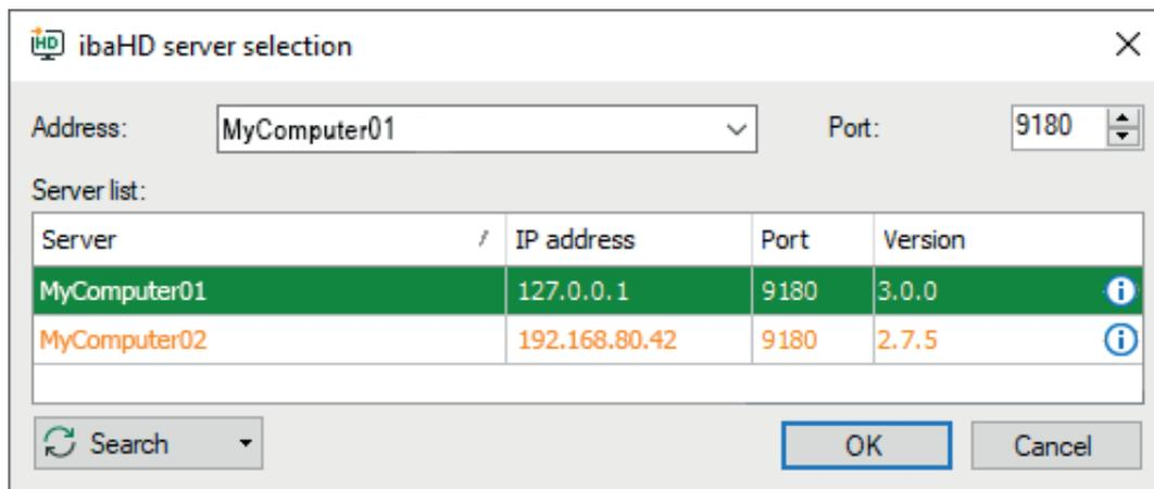
Use the <Search> button to scan the network for active HD servers and select a server from the table or type in a server address. Click the <OK> button to connect to the *ibaHD-Server*. If the HD signal tree has not been visible yet, it will be shown automatically in the *ibaPDA* client.
