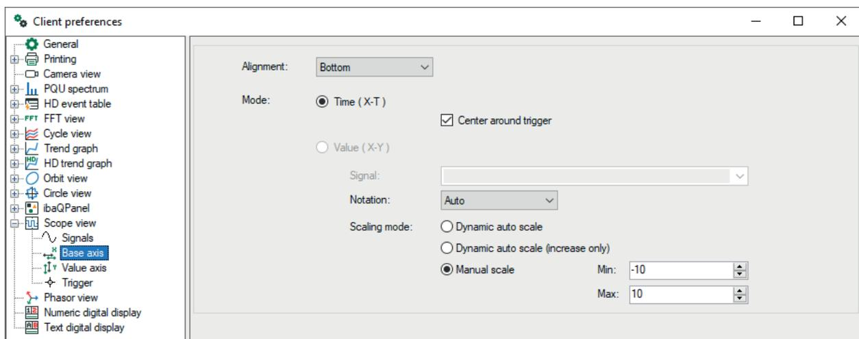
The base axis is always the horizontal axis in a scope view.
