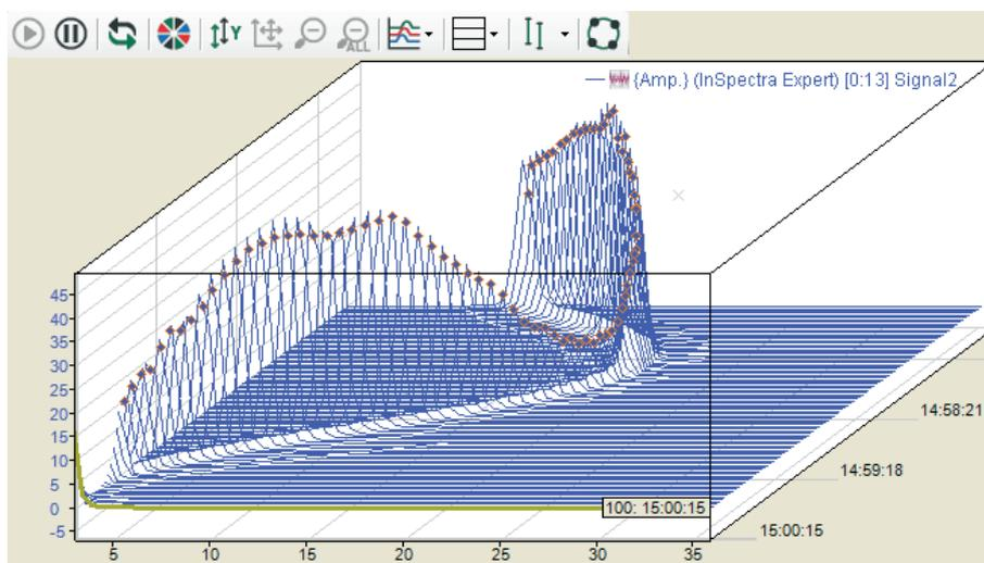
In the above figure, you can see the results of the last 100 calculations and it is clearly visible how the spectrum changed in the course of time.
