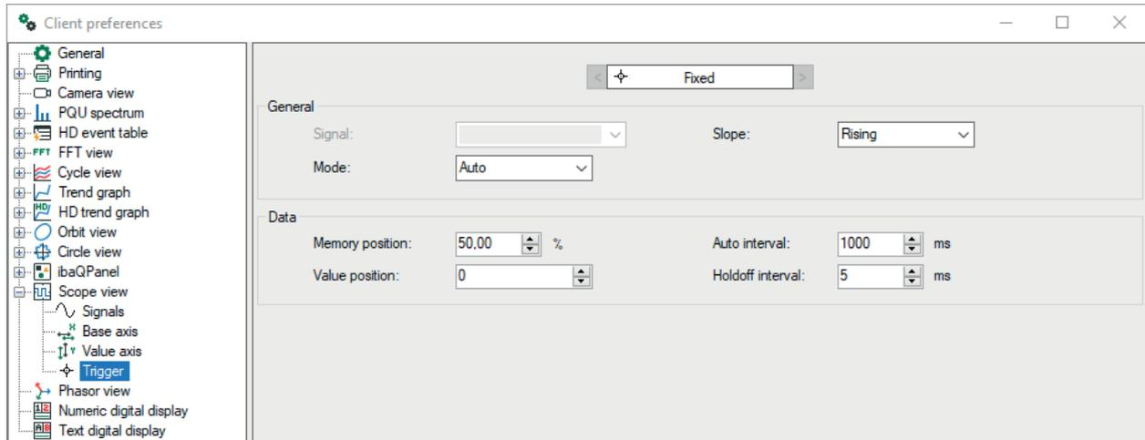
In the "Preferences" dialog, you can set the general options for the trigger, such as the mode (normal, single, auto and auto level) and trigger edge (rising, falling, both and alternating). The signal selection is disabled. The signal for controlling the trigger can be selected in the view's "Properties" dialog.
