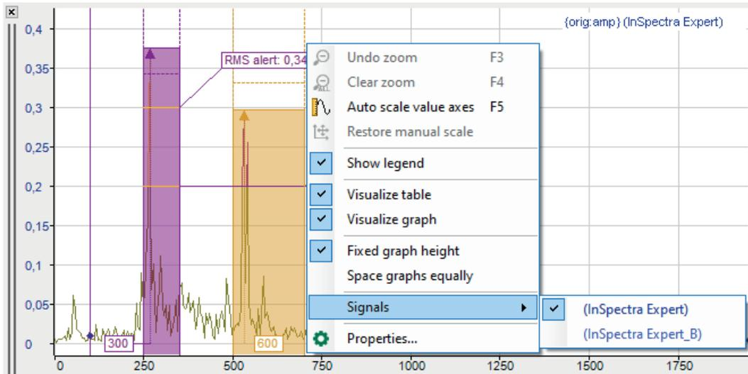
If there are several spectra in the display, individual display properties can be assigned to every spectrum.
