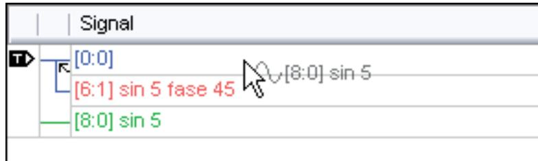
The signal table's height can be adjusted. When moving the mouse to the top of the table, a resize icon appears. To auto-size the table, double-click if the resize icon is visible.
