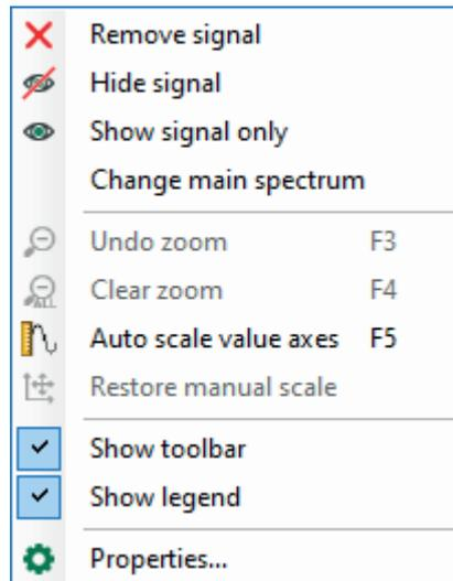
Clicking on “Remove signal” removes the corresponding signal. Clicking on “Hide signal” hides the signal and shows the signal name transparently. The signal is only temporarily hidden and can always be displayed again. By clicking on “Show signal only” in the context menu, only the selected spectrum remains in the display and all other spectra are hidden. Clicking on “Change main spectrum” makes the selected spectrum the main spectrum.
