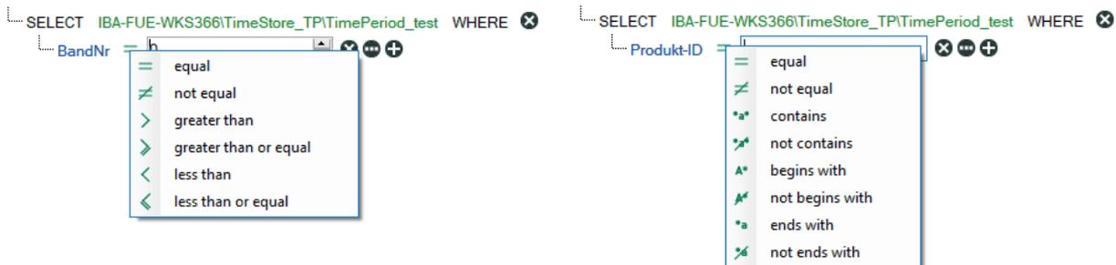
Behind the elements in the query, there are different buttons which you can use to extend or modify the query:
