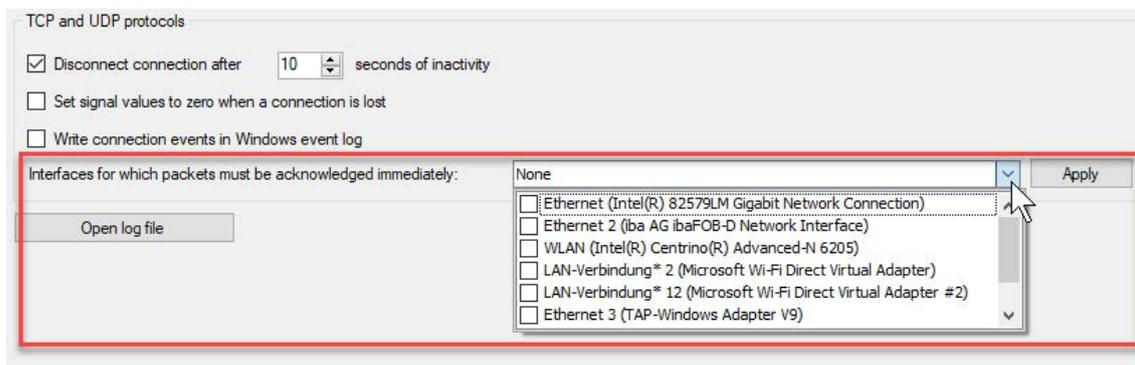
Thus, the parameter "TcpAckFrequency" (REG\_DWORD = 1) is created in the registry path of the selected network adapters:
