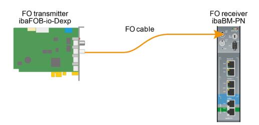
The example refers to a point-to-point connection with an FO cable of type 62.5/125  $\mu$ m. The light wavelength used is 850 nm.
