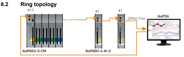
Up to 15 devices can be connected to a ring. Configuration and process data are transmitted in the ring.
