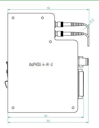
Dimensions ibaPADU-4-AI-U with cable (Dimensions in mm)
