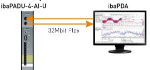
The device is connected to the ibaFOB-D card in the ibaPDA PC via a bidirectional FO line to transfer configuration and process data. ibaPDA detects automatically the connected device.
